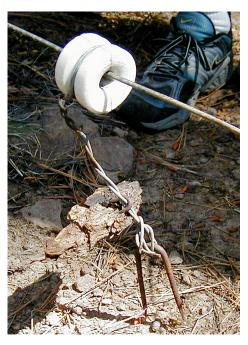
Fig. 4-17. Three-Inch Staple. The three-inch staple that once held this medium round split knob to the tree in Twomile Canyon has pulled off allowing the line to fall. (GPS waypoint TM4)
