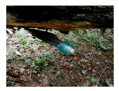
Fig. 5-8. Topless Hemingray on Fallen Snag. This Hemingray site is located along the old road that once crossed upper Frijoles Canyon between the plateau and the Valle Grande. The road and line crossed the southeastern corner of the Baca Location and once connected the Pajarito Plateau to the Jemez Mountains. The artifact exhibits the typical problems of the Hemingray glass. The glass dome cracks and breaks off when it freezes, and the wood bracket splits as the tree grows. (GPS waypoint UF10)
