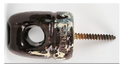
Fig. 4-21. Post-style Insulator. This insulator, designed to screw directly into the telephone pole, was the type used along a later section of telephone line that dropped into Los Alamos Canyon from the Army barracks on the canyon's north side.
