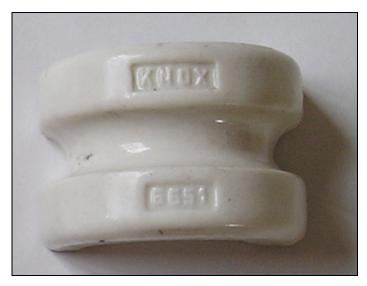
Fig. 4-12. Large Oval Knox Insulator Half. The KNOX trademark is embossed in a recessed rectangle on the upper outside edge, the style number 6651 on the lower outside edge. (GPS waypoint PO7)
