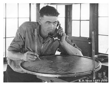
Fig. 2-10. Fire Guard Phones in Fire. The guard uses an Osborne fire finder to get the bearings of possible fire. He then telephones the information to the district ranger, who uses information from two or more fire towers to determine the fire location and to organize a fire fighting crew. (Photo: U.S. Forest Service)
