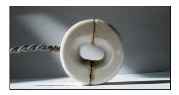
Fig. 4-9. Large Round with Oval Center Hole. The oval shape of the center hole was a modification in design to prevent the telephone wire from getting caught and pulling at the joint of the two halves.
