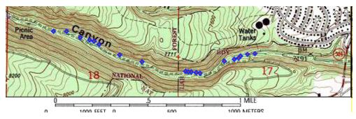
Fig. 5-17. Telephone Line along Road to Los Alamos Reservoir. These diamonds mark the tie trees with brown oval knobs or metal brackets. The tie trees follow along the current Reservoir Road, located south of the old trail. Several of the brown oval knobs are embossed with "NAT" for the National Forest. The metal pins were possibly part of a later update of the line.
