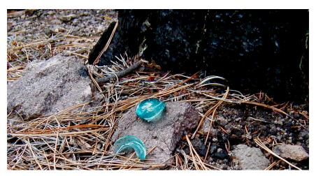
Fig. 4-3. Popped Top and Split Bottom. These two photos demonstrate the problems with the glass insulator and wood bracket. The insulator top has apparently popped off due to freezing and the end of the bracket has split and broken away as the girth of the tree expanded. This ponderosa is located on West Jemez Road. (Geographic positioning system [GPS] waypoint WJ1)
