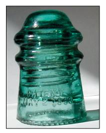
Fig. 4-2. Hemingray No. 9. This small blue glass insulator was the type first used on the Jemez Forest Reserve in 1906. Note the drip points around the bottom and the threads that allowed the insulator to be screwed onto the bracket.
