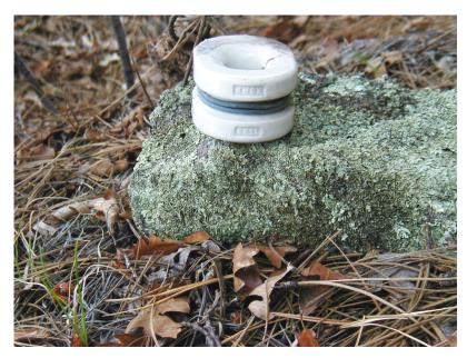
Fig. 5-34. Knox on Branch-line to Pajarito Cabin. This oval split knob was found along the line built around 1939 to the Pajarito Ranger Cabin. (GPS waypoint PO7)
