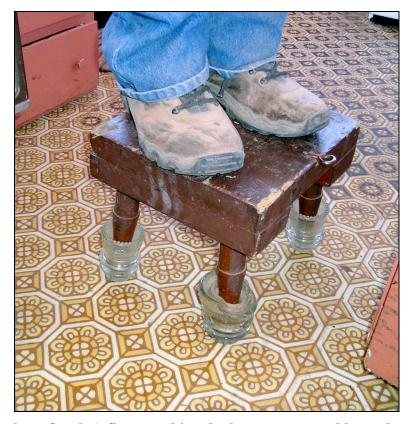
Fig. 2-16. Lookout Stool. A fire guard in a lookout tower would stand on an insulated stool for protection during electrical storms. The stool has four glass telephone insulators screwed onto the feet of the stool. Frank Gonzales demonstrates standing on the stool at Cerro Pelado Lookout.
