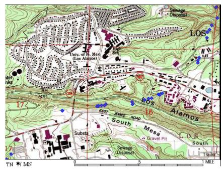
Fig. 5-27. New Crossing of Los Alamos Canyon. The blue diamonds mark tie trees along the relocated line that crossed Los Alamos Canyon by dropping down the Dead Man Trail on the north side and angling up the Duran Road on the south.
