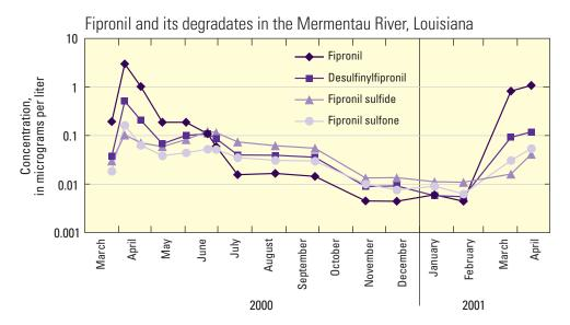
**Figure 5–14.** Concentrations of the insecticide fipronil and its degradates in the Mermentau River (Acadian–Pontchartrain Drainages) peaked in March or April, following applications. Although fipronil dominated the total concentration of fipronil compounds during the high-use period, concentrations of its degradates were greater during the rest of the year (Demcheck and others, 2004).
