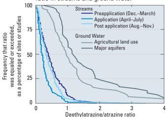
Figure 5–16. The ratios of deethylatrazine to atrazine concentrations—which increase with the transformation of atrazine to deethylatrazine—increased with increasing residence time in the hydrologic system. (Ratios were computed from µg/L concentrations for all NAWQA stream and ground-water samples in which both compounds were detected.)
