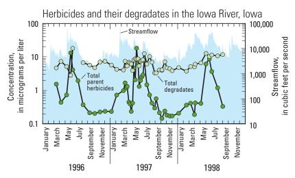
**Figure 5–13.** The summed concentrations of the parent herbicides atrazine, cyanazine, acetochlor, alachlor, and metolachlor in the lowa River (Eastern lowa Basins) rose and fell in response to spring applications, whereas the summed concentrations of their degradates remained relatively steady and at higher levels throughout most of the year (Schnoebelen and others, 2003).
