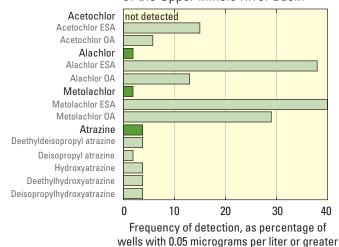
Figure 5–15. In ground water of the Upper Illinois River Basin, degradates (light bars) were generally detected more frequently than parent compounds (dark bars) for the acetanilide herbicides (acetochlor, alachlor, and metolachlor), but at comparable frequencies for atrazine (Groschen and others, 2004).
