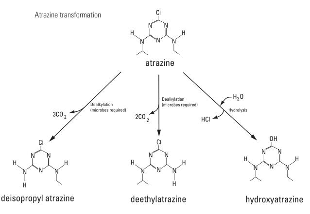
**Figure 5–12.** Atrazine transforms to three primary degradates (although there are others as well), one of which—deethylatrazine—was routinely measured by NAWQA. Two of these transformation reactions require microbes, resulting in the formation of deethylatrazine and deisopropyl atrazine. The third is hydrolysis, an abiotic reaction with water that produces the degradate hydroxyatrazine.
