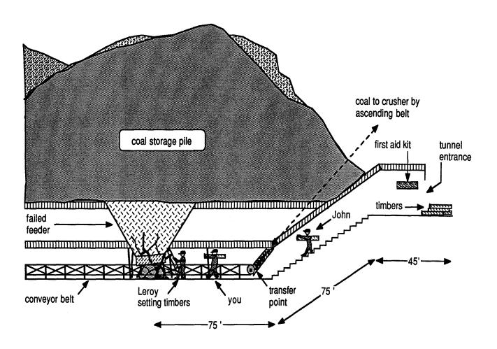
Figure 1: Schematic of tunnel under main stock pile (not to scale)
