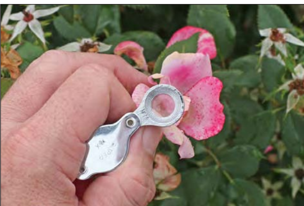
Figure 21. A hand lens provides useful magnification for field diagnostics. (Photo by Joe Boggs)
