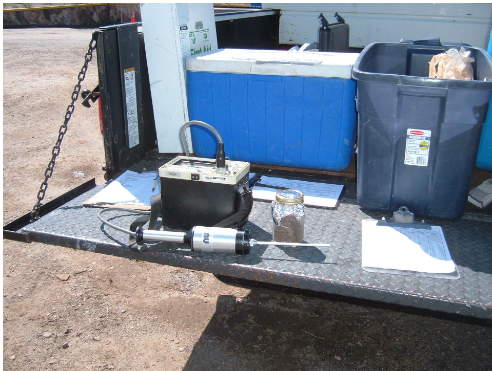
Figure B-16 Photoionization detector used for headspace readings. Note mason jar with aluminum foil.
