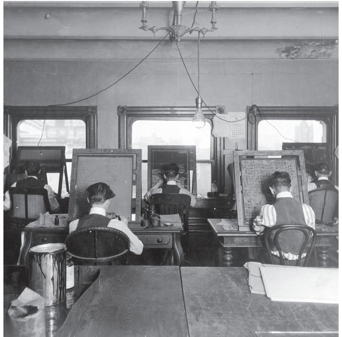
Figure 2. USGS employees scribing copper plates for map production in 1917.
