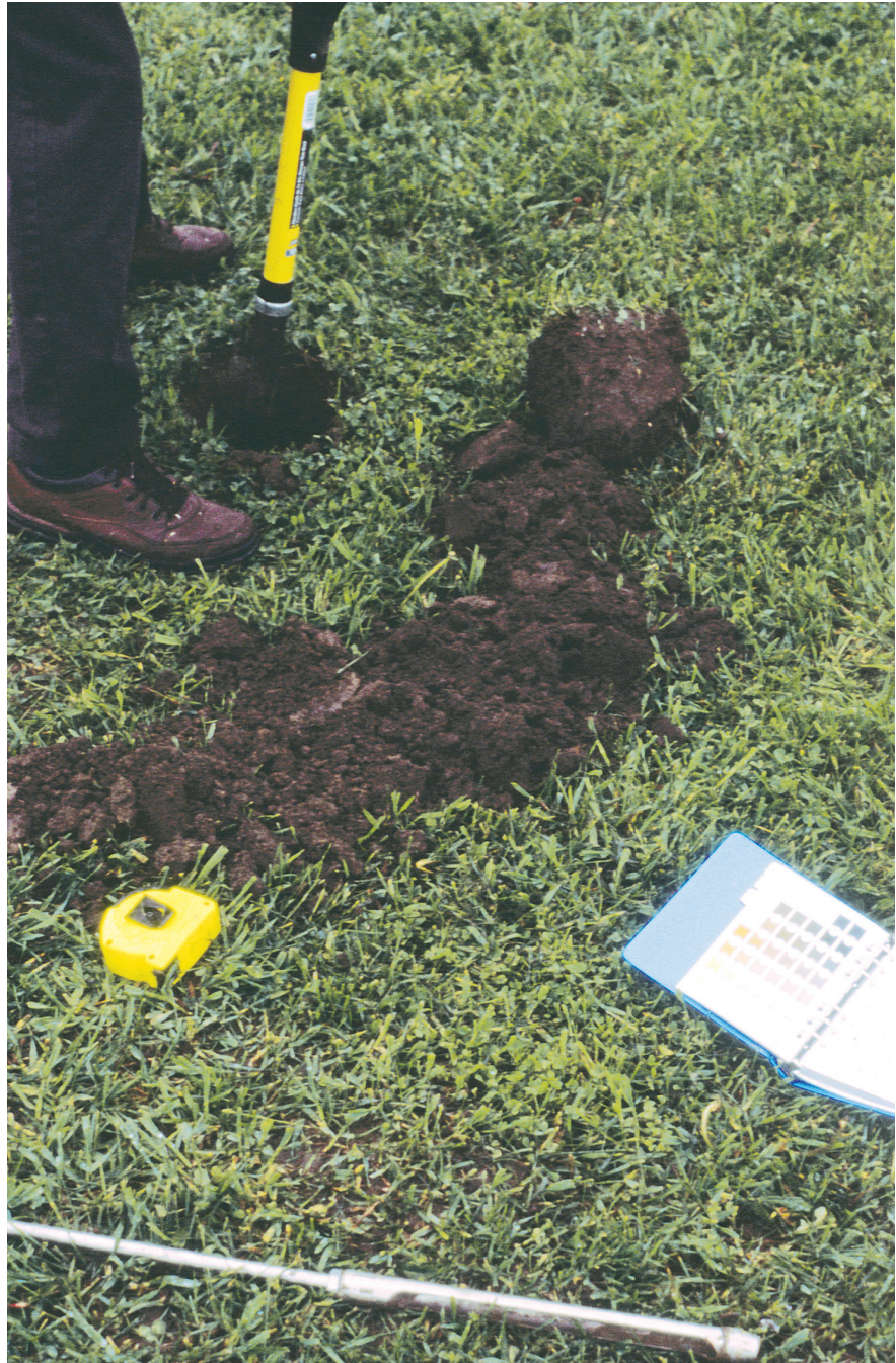
Figure 11. Detailed descriptions of the identified soil types on the lot are generated from several soil cores. Soil is lifted out of a small hole with a spade or auger and placed on the ground in order. Evaluator observes and notes color patterns, texture, structure and consistence of each soil horizon.
