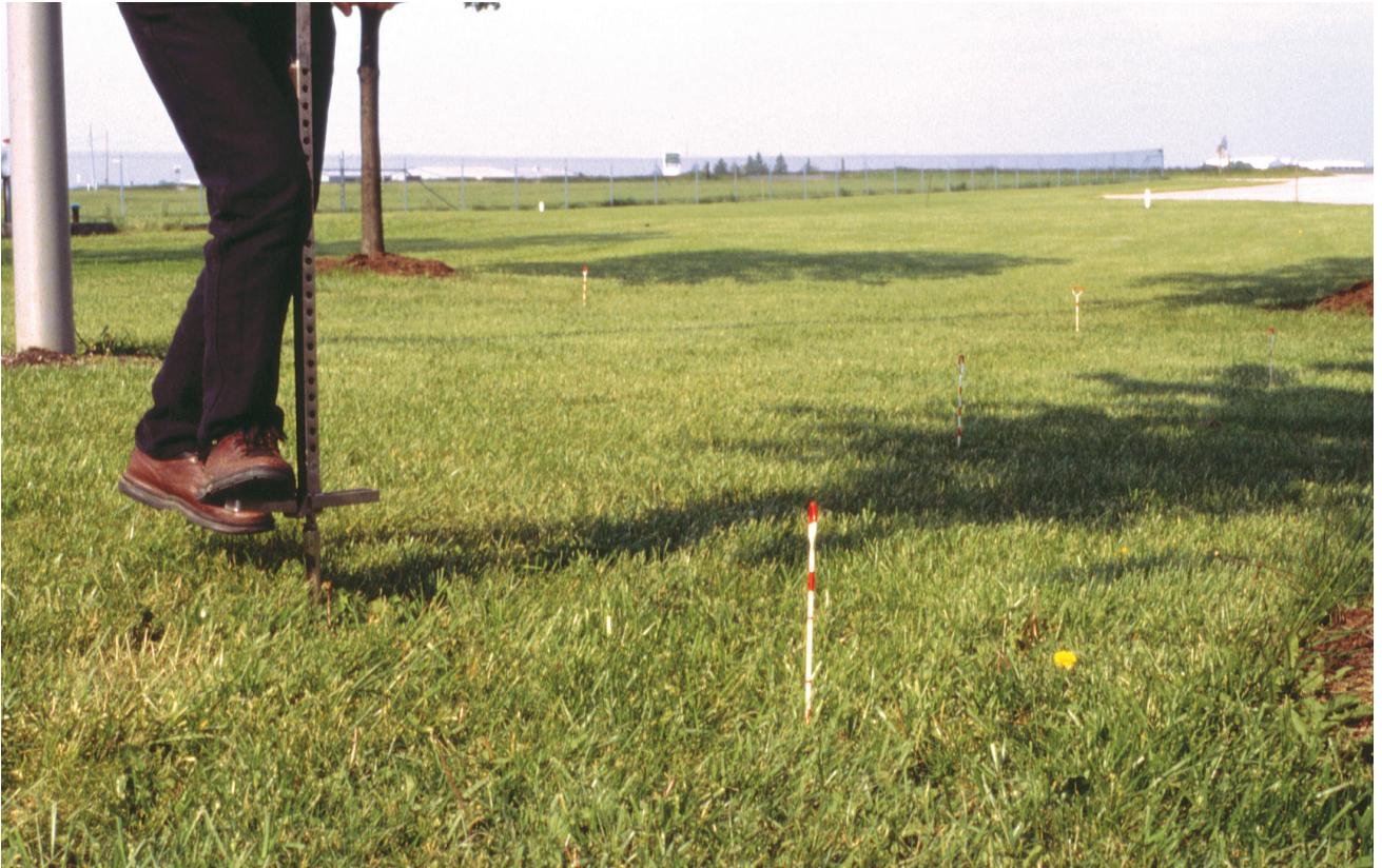
Figure 10. Using a soil probe, soil is examined on either side of the pins to confirm soil differences. Pins are moved as necessary.
