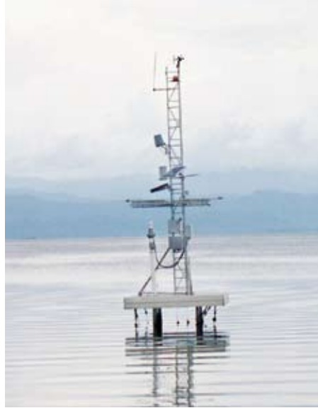
An automated data station records hourly values of oceanographic and meteorological data, including water level, rainfall, and solar and quantum radiation. Hourly sea temperature is also recorded at seven remote sites in the surrounding area.
