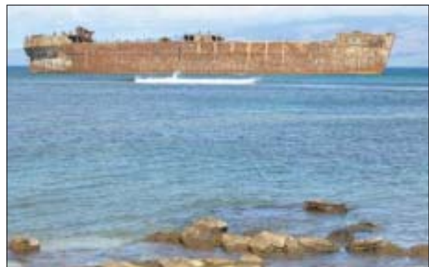
Figure 239. This U.S. Navy steel-reinforced concrete vessel has been hard aground off Shipwreck Beach, Lanai since the 1950s (Photo: Hans van Tillburg).
