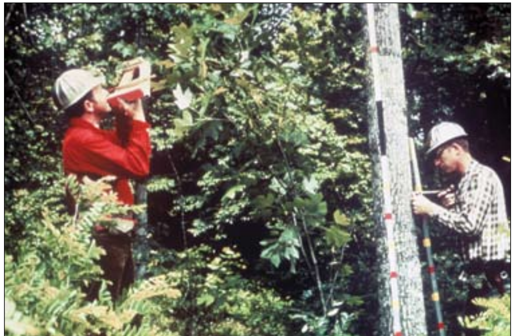
Photo 8.—Noel Cost measures a tree with the McClure caliper while John Nesbit measures bark thickness, Virginia, circa 1966.
