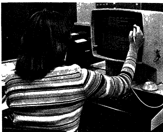
A computer operator uses a "light pen" attached to a cathode ray tube to interact with the computer system
