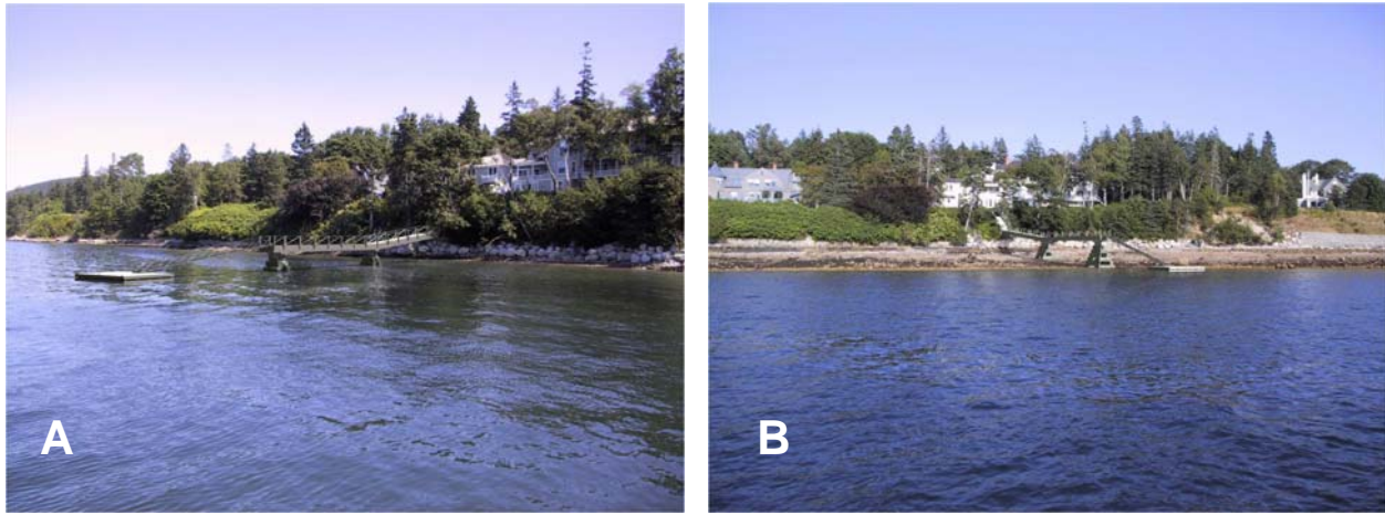
Figure 3. Computerized images of a proposed dock in Somes Sound, Maine. These images provide examples of the way that Visual Impact Simulation can be used to review proposed projects. The dock and float in the center of the photographs do not presently exist; they have been superimposed on the existing background through the use of a computer program. “A” shows the dock at high tide and “B” shows the exposed cribs at low tide. These images were developed by John Gutwin for the using PhotoModeler® and LightWave®, used with permission.
