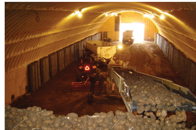
Figure 4—Here, potatoes move on a conveyor belt into a storage cellar.
