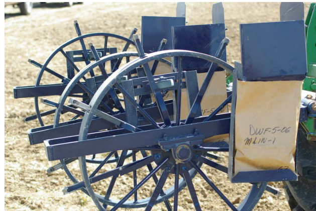
Figure 6—Mechanical wheel soil samplers like this one were used during the PCN survey in 2006.
