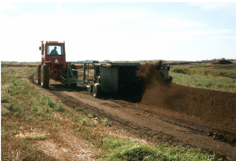
Plate 3. A poultry manure windrow composting operation. Pictured here is a low cost tractor-pulled windrow turner which serves to mix and aerate the compost, and ensures the cooler parts of the outside of the windrow are exposed to hotter conditions in the interior to ensure pasteurisation occurs.
