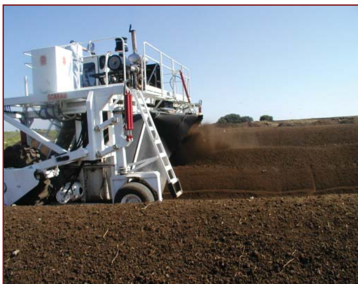
A scarab mixes the dairy manure during the composting process to aerate the windrow which ensures proper composting.
