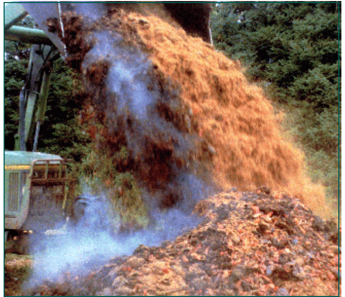
Turning heating a windrow with front-end loader.
