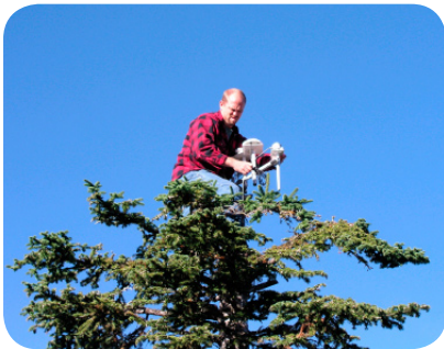
Above (top): Radiometers installed in headwater streams to determine the effect of forest harvest and BMPs on stream heating.
