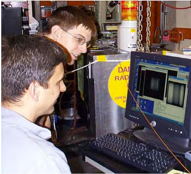
Fig. 33. Stuart Miller (front) and Jeff Bunn examine a neutron image of steel tubes which had been subjected to deformation.
