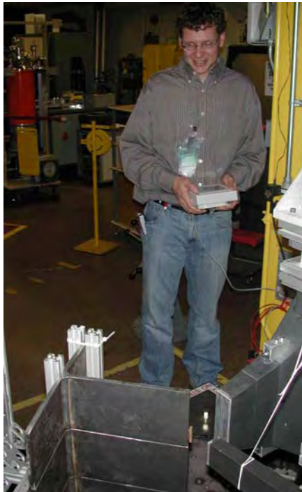
Fig. 30. Eric Johnson of John Deere positioning the welded “T” plates for neutron diffraction at the Engineering Diffractometer at High Flux Isotope Reactor (HFIR), Neutron Residual Stress Facility 2 (NRSF2).
