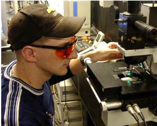
Fig. 15. Tim Jochum collecting Raman spectra on his \beta -eucryptite sample.
