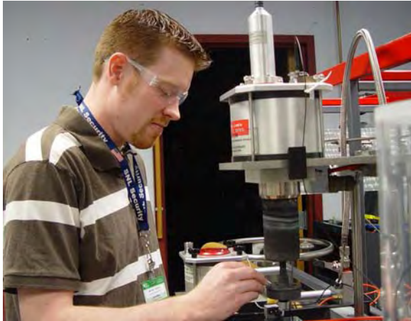
Fig. 38. Michael Teague of MUS&T working at the TTPUC's laser flash thermal diffusivity
