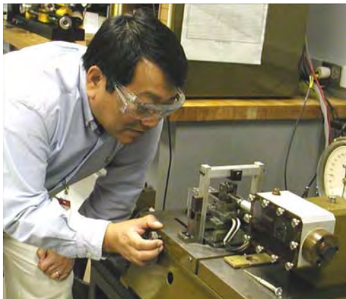
Fig. 39. Prof. Linan An conducting a ball-on-flat friction and wear test.
