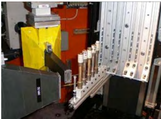
Fig. 34. Tension- and torsion-deformed steel tubes mounted on NRSF2 for measurement of the hoop strains.
