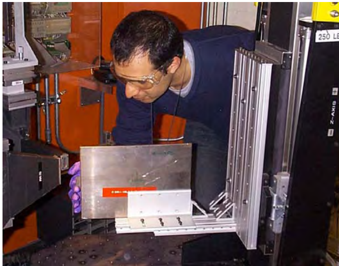
Fig. 26. Dr. Villasana of Metalsa mounts a plate sample for through thickness strain mapping as a function of distance from the hole along a line transverse to the rolling direction of the plate.
