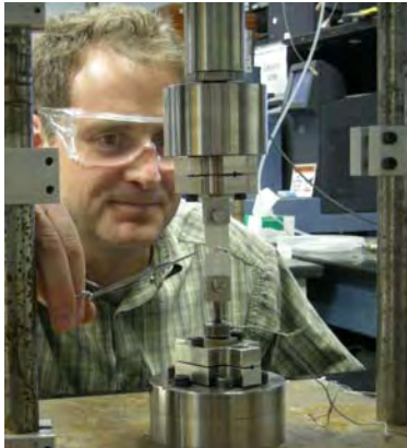
Fig. 19. David Haack testing unused single carbon fibers under tension.
