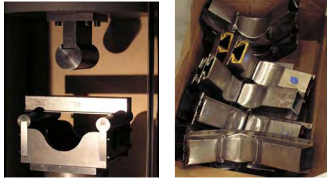
Fig. 16. 3-point bend test equipment (left) and crushed bend specimens after successful testing (right).
