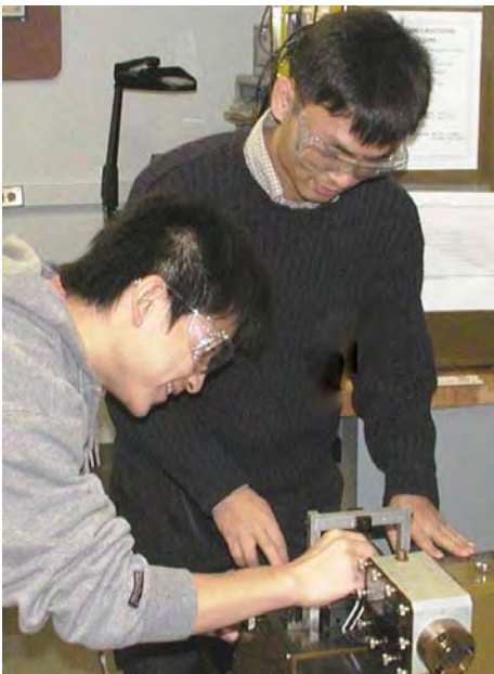
Fig. 35. Prof. Park (right) and Mr. Li adjust a specimen on the reciprocating wear test system.
