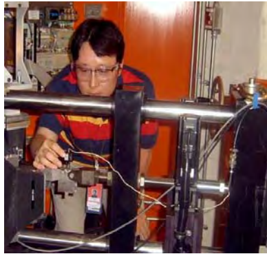
Fig. 33. Sooyeol Lee sets up in situ loading for neutron diffraction measurements.
