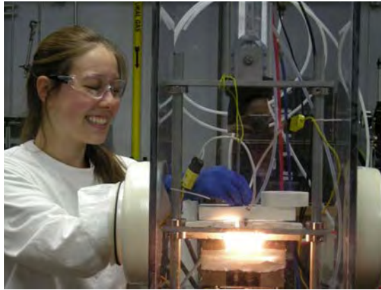
Fig. 10. MSU student Jennifer Ni using the infrared (IR) set-up to thermal cycle thermoelectric materials.
