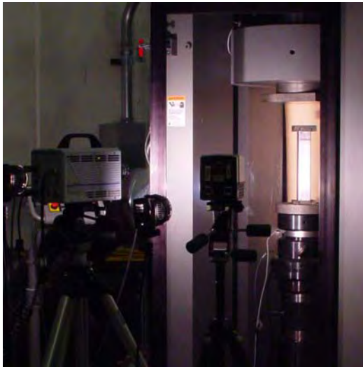
Fig. 12. High-speed and thermography cameras ready for high-rate testing of steel crush tubes.
