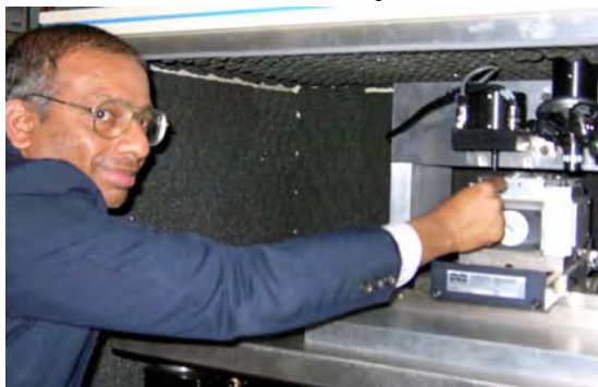
Fig. 26. Professor Tirumalai Srivatsan uses an HTML nanoindenter to measure elastic modulus and hardness of boron carbide samples.
