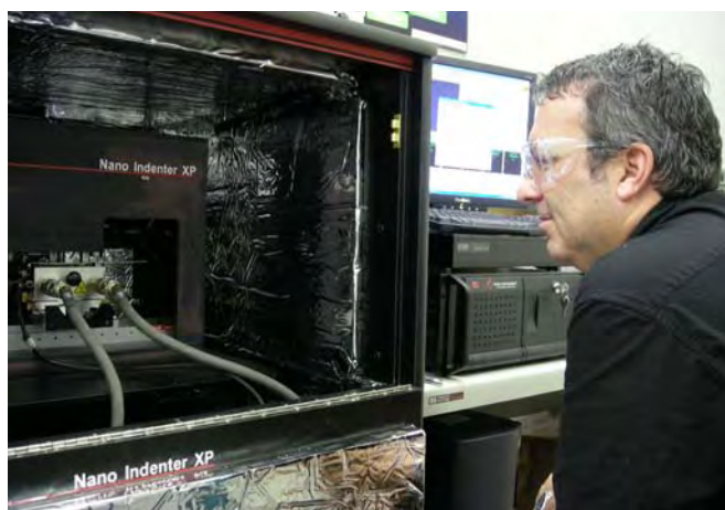
Fig. 28. David Goldsby monitors nanoindentation measurement of quartz creep.
