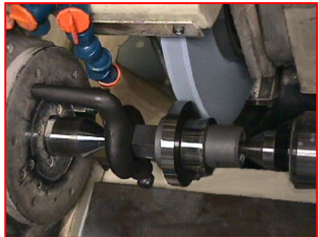
Figure 2-1. The Weldon cylindrical grinder is used to test combinations of coolants and grinding wheels by grinding Type 52100 steel specimens.
