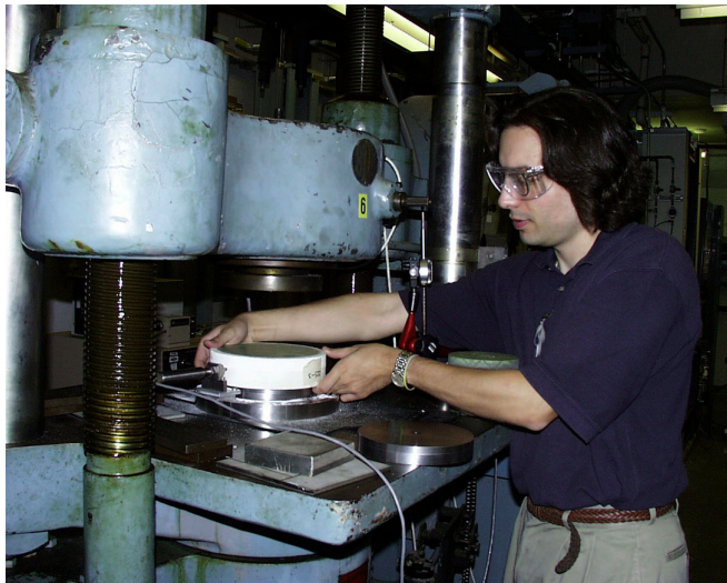
Fig. 3-4. Siemens-Westinghouse engineer Eric Carelli preparing the section of an all-oxide combustor liner for an internal pressurization test.
