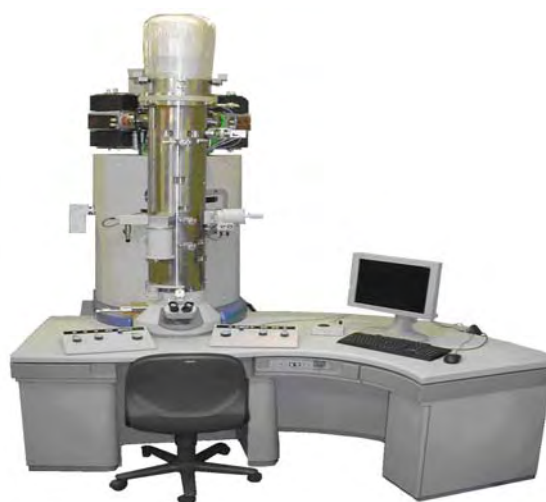
Figure 54. The newly delivered HF-3300 cold field emission TEM/STEM instrument. Douglas Griffith (seated left) hosted HTML's Karren More and Jane Howe at the Hitachi Naka factory for pre-shipment testing.
