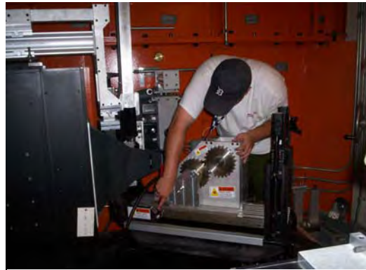
Fig. 35. Static Load Application Device is prepared for use at NRSF2.
