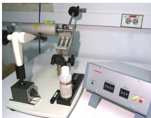
Fig. 51. Ball cratering system with multi-axis specimen holder and control unit.
