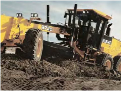
Fig. 28-a). John Deere road grader. The grader gear controls the blade, which moves the earth. Fig. 28-b). Using a lift plan, (L to R) Barton Bailey, Camden Hubbard (ORNL) and Tom Mauger (John Deere) lift a gear.
