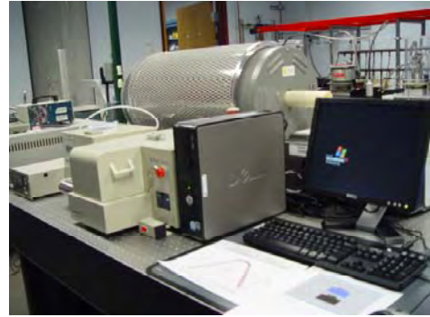
Fig. 56. ULVAC LaserPit system installed at TTPUC for thin film studies.
