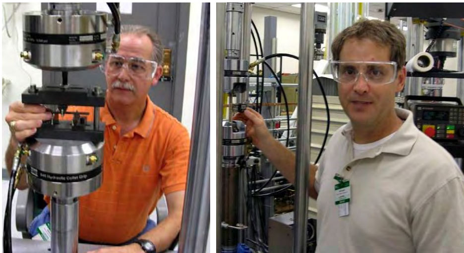
Fig. 6. MIT’s Mark Janney (left) and David Haack conduct tensile and flexural tests on composites manufactured with 3-DEP process.
