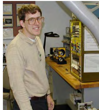
Fig. 46. Prof. Jackson at the Plint TE77 wear testing and reciprocating friction machine used to study biomimetic surfaces. Driving mechanism and specimen fixtures at lower right.
