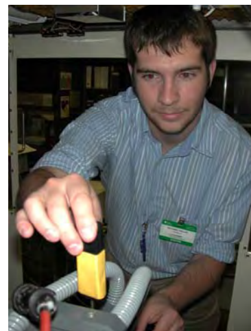
Fig. 26. Nate Phillips adjusts sample height on the PTS rotating anode diffractometer.
