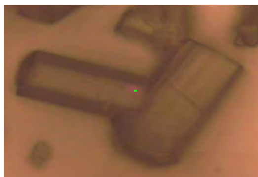
Fig. 12. A 30 by 30 \mu\text{m} stress map (left) was obtained from a region on the sample where two AlN grains were connected (above). At the interface, the AlN Raman peak shifts to lower frequency (blue color), suggesting a tensile stress.
