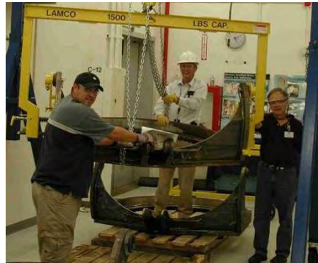
Fig. 28-a). John Deere road grader. The grader gear controls the blade, which moves the earth. Fig. 28-b). Using a lift plan, (L to R) Barton Bailey, Camden Hubbard (ORNL) and Tom Mauger (John Deere) lift a gear.
