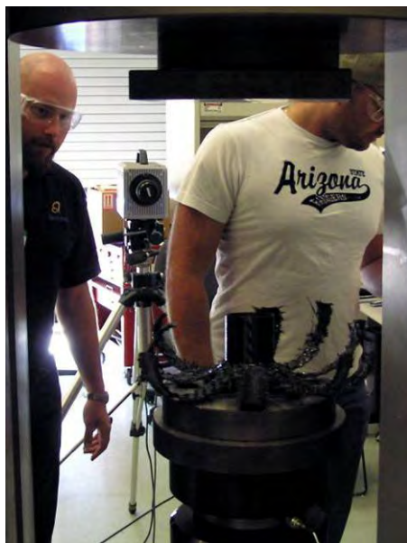
Fig. 4. Quickstep™ engineers Aaron Brighton and Dale Brosius retrieving a composite tube after a crush test using ORNL's TMAC.
