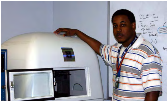
Fig. 22. FSU graduate student Steve Downey using the Hysitron nanoindenter to measure the hardness and elastic properties of M316LN.
