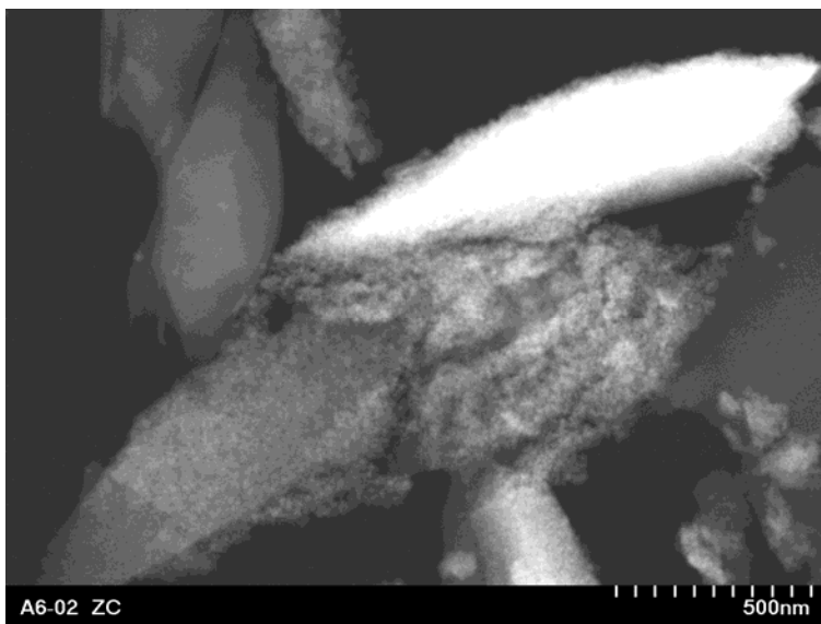
Fig. 17. A z-contrast STEM image shows iron oxide (brighter area) deposited on porous Si (darker objects).
