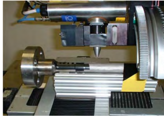
Fig. 30. At left, Pei-Yuan Cheng monitors the data collection process. At right, the 304 stainless steel sample with a socket weld set up for hoop strain measurement.
