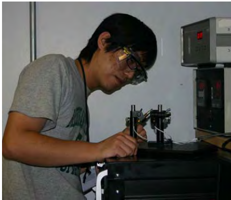
Fig. 9. MSU graduate student Fei Ren using the RUS to determine the elastic properties of thermoelectric materials.
