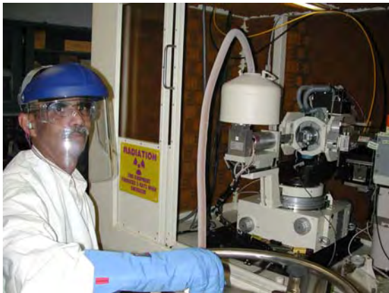
Fig. 32. Dr. Jag Kasichainula fills the Dewar on the detector on the PTS rotating anode unit with liquid N 2 .
