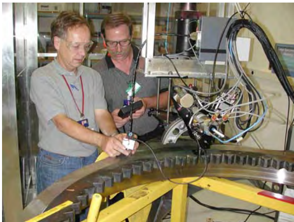
Fig. 29. Tom Mauger (left) and Kent Schumacher (John Deere) adjust the height of ORNL’s large specimen x-ray unit by adjusting its height using a remote control cabled to a Z-motor. The x-ray unit, a TEC 1640, is suspended on a gantry with x, y and z movements available. The yellow cart holds the gear with the “top” side up. Figure at right depicts the residual stress distribution in one of the gears.
