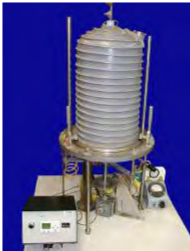
Fig. 2-4. High-temperature hardness tester vacuum chamber and lifting apparatus (left); effects of temperature on the Vickers microindentation hardness of Stellite 12 (right).
