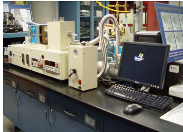
Fig. 6-4. The ULVAC ZEM-2 system installed at the HTML.
