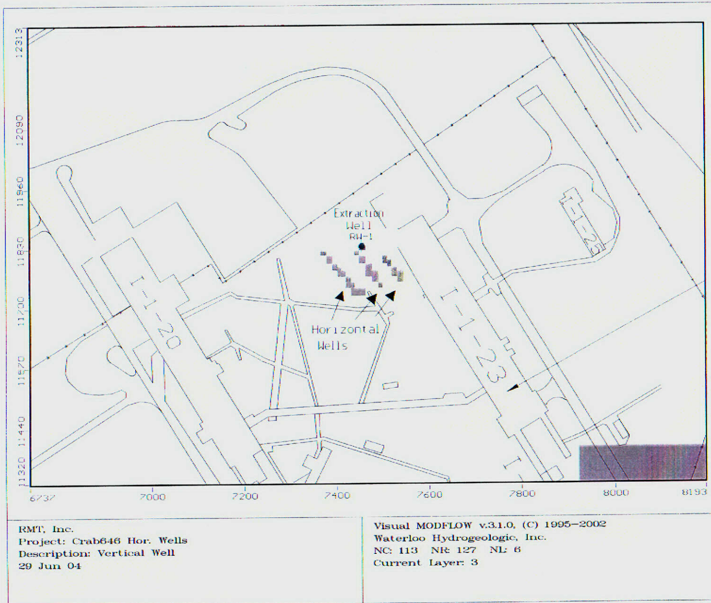
Location of horizontal wells, simulated as drains, Alternative C, I-1-23
