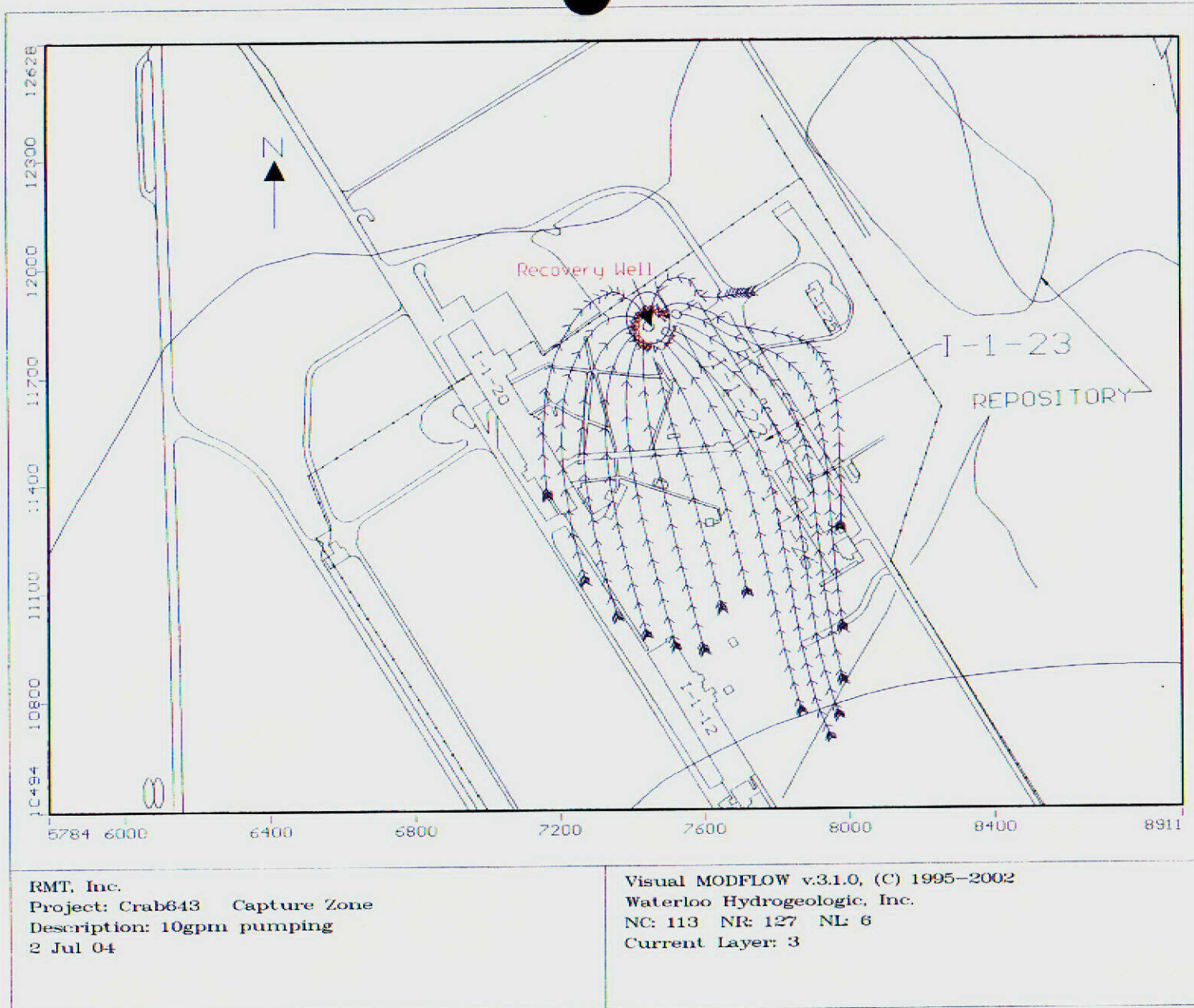
Capture Zone of Extraction Well, 10 gpm, I-I-23
