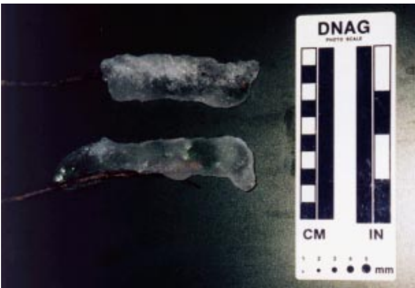
Figure 22 (cont'd). Ice accretions with measured or estimated uniform ice thickness.
