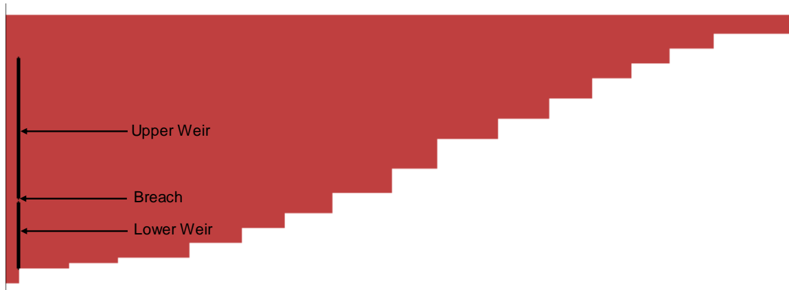
Figure B-2: East Canyon Reservoir W2 model internal weirs
