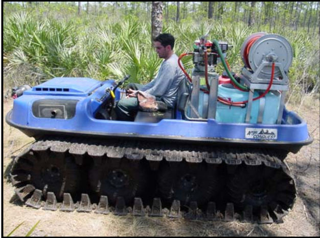
Figure 17. Tracked swamp buggy equipped with a 25 gallon sprayer used by private contractors to reach Old World climbing fern infestations in south Florida.
