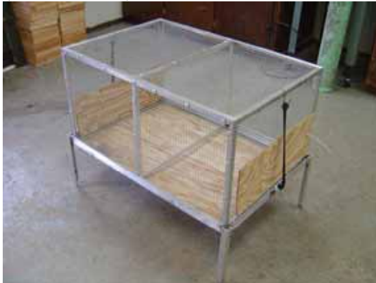
Fig. 7. Standard closed bottom mussel excystment cage deployed in L. higginsii recovery project
