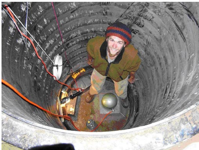
Mike Busby of the USGS's Albuquerque Seismological Laboratory stands astride seismic sensors in the 10-foot-deep vault of station EGAK in Alaska near the Yukon border. EGAK is one of over 100 stations in the Advanced National Seismic System (ANSS) ‘backbone’ network.
