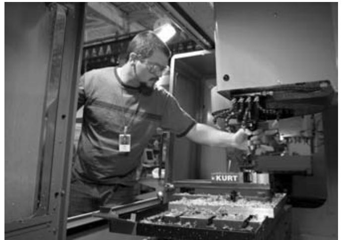
Machinists change worn cutting tools on computer-controlled machines.
