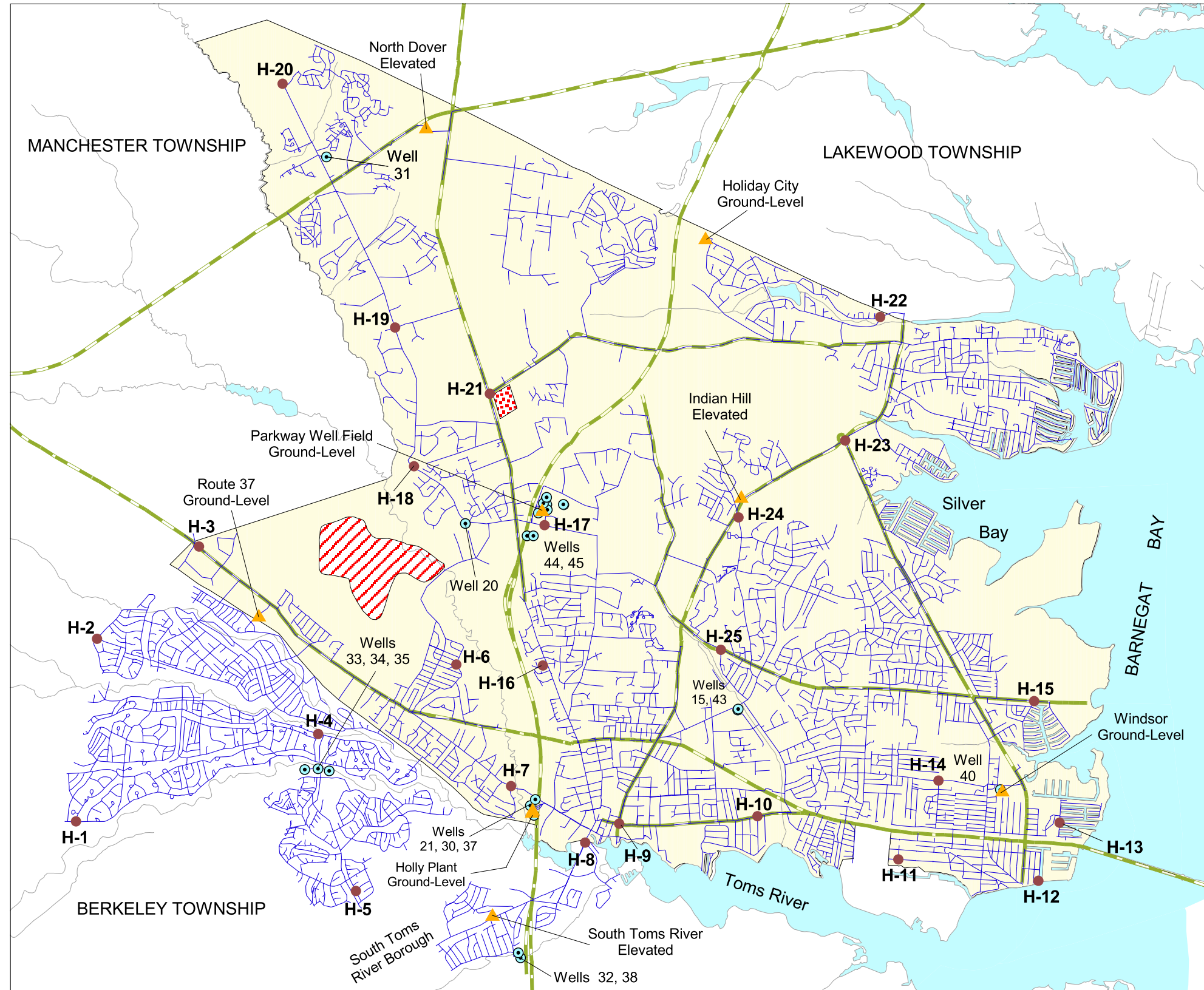
PLATE 4. LOCATIONS OF PROPOSED TEST HYDRANTS FOR COLLECTING SYSTEM-WIDE PRESSURE DATA DOVER TOWNSHIP AREA, NEW JERSEY
