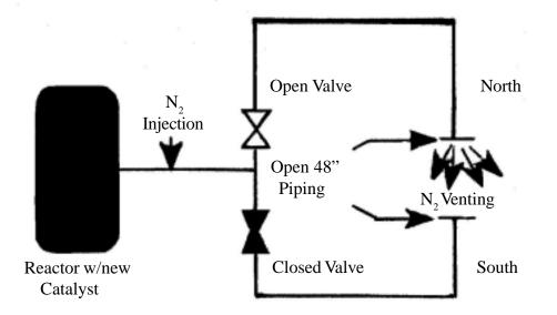
Note: Actual process/piping significantly more complex.  $N_2$  injection point 150° and several stories in elevation from pipe opening.
