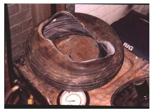
Picture depicting damage to tire that occurred during attempt to inflate a mismatched tire and rim
