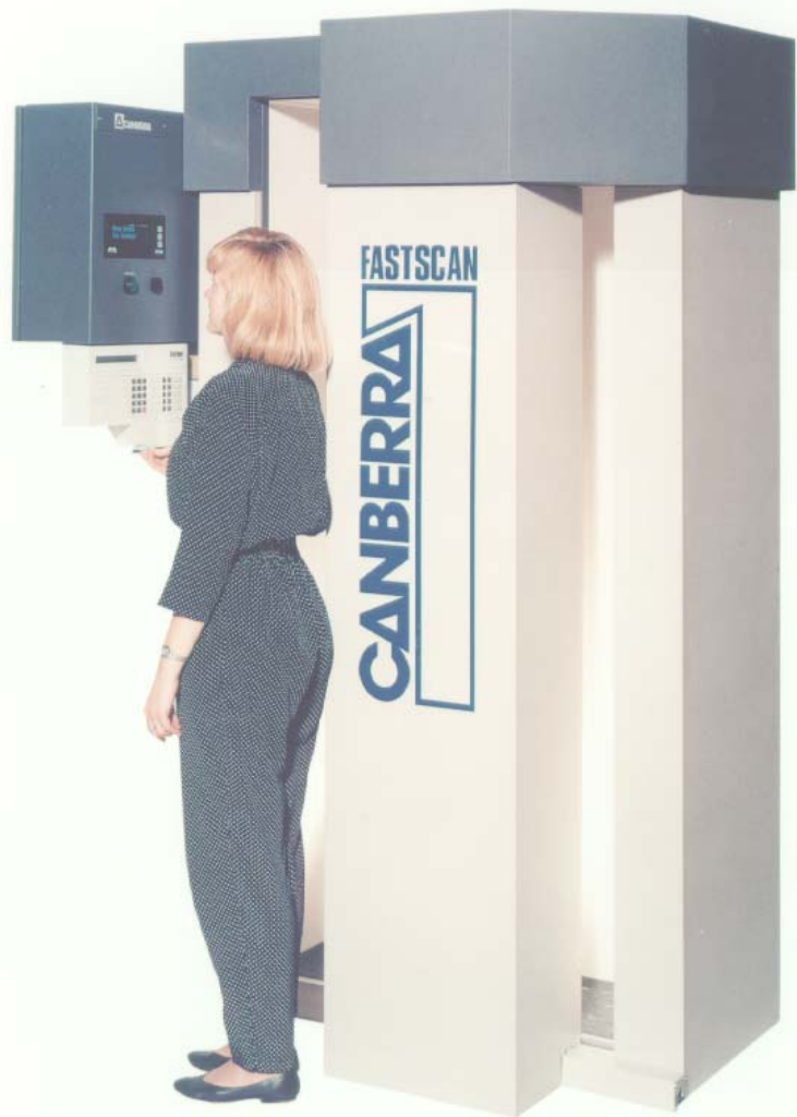
Figure 2-2. Whole Body Counter. The linear geometry NaI based WBC pictured here is designed to maximize sensitivity and accuracy for internally deposited fission/activation products such as isotopes of Cs and Co. (Photograph courtesy of Canberra Nuclear/Packard BioScience Co.)
