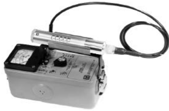
Figure 2-6. Geiger-Mueller Counter with an Energy-compensated Gamma Probe. (Photo courtesy of Ludlum Measurements, Inc.)
