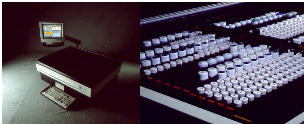
Figure 2-5. Liquid Scintillation Counting (LSC) System. Shows system (left) and closeup view of sample vials to be loaded (right). (from Canberra/Packard Bioscience Co.)
