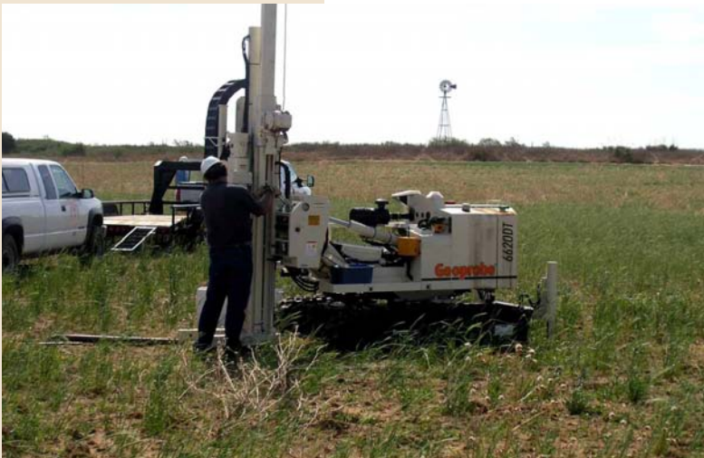
Drilling in the Ogallala aquifer in Kansas to determine the groundwater supply.
