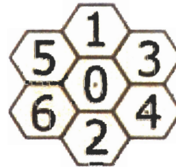
Figure 1. Anode pad arrangement for charge sharing measurements (part of a larger array using the same geometry). Center to center spacing is 5 mm.
