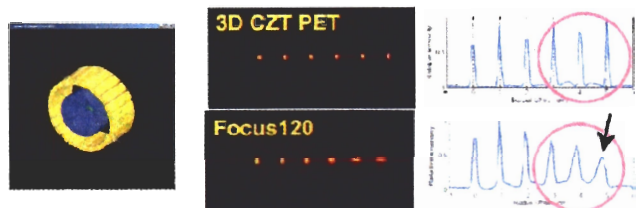
Figure 1. Scanner geometry (left), point-source images across FOV (middle), and profiles through images (right).
