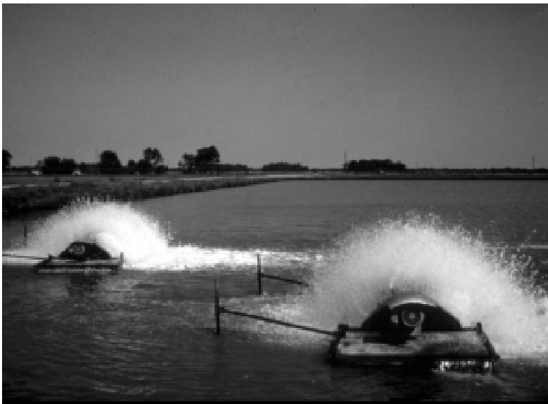
Aerators increase oxygen levels in pond water. Courtesy of Louisiana Cooperative Extension Service.
