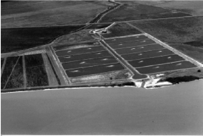
Austwell Aqua Farm's 12 five-acre ponds are located on a shallow secondary bay on the Texas Coast — a typical design for Texas' coastal shrimp farms. Photo courtesy of Texas Parks and Wildlife Department.
