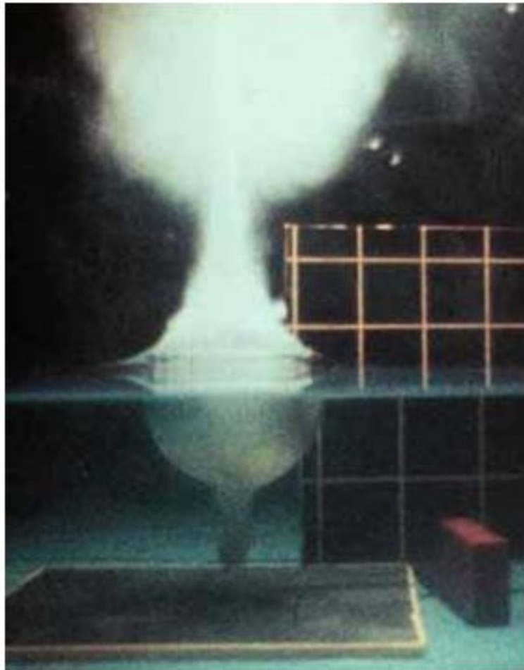
Figure 2 – Gault and Sonnet results for a 0.635 cm diameter Aluminum Projectile moving at 2.5 km/sec and for a 0.3175 diameter Pyrex Projectile moving at 2.32 km/sec
