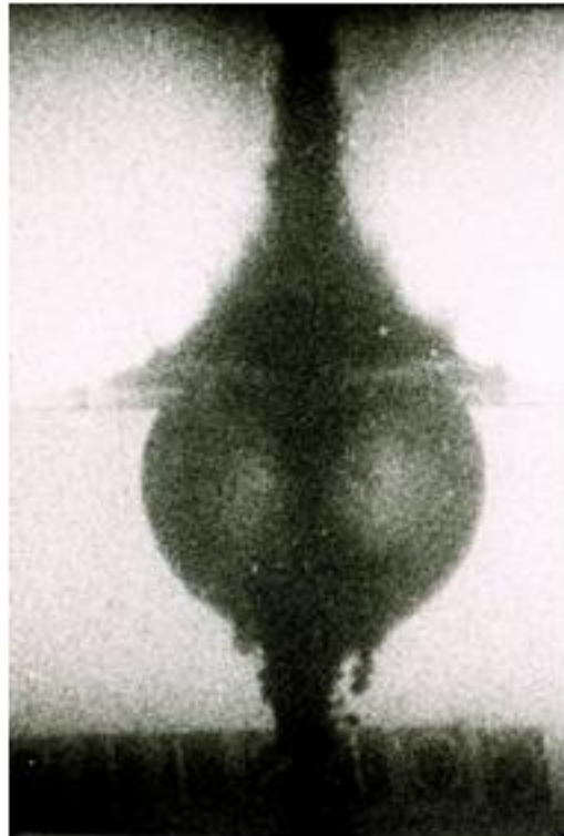
Figure 1. Gault and Sonnet results for a 0.25 cm diameter Aluminum Projectile moving at 1.8 km/sec impacting water.
