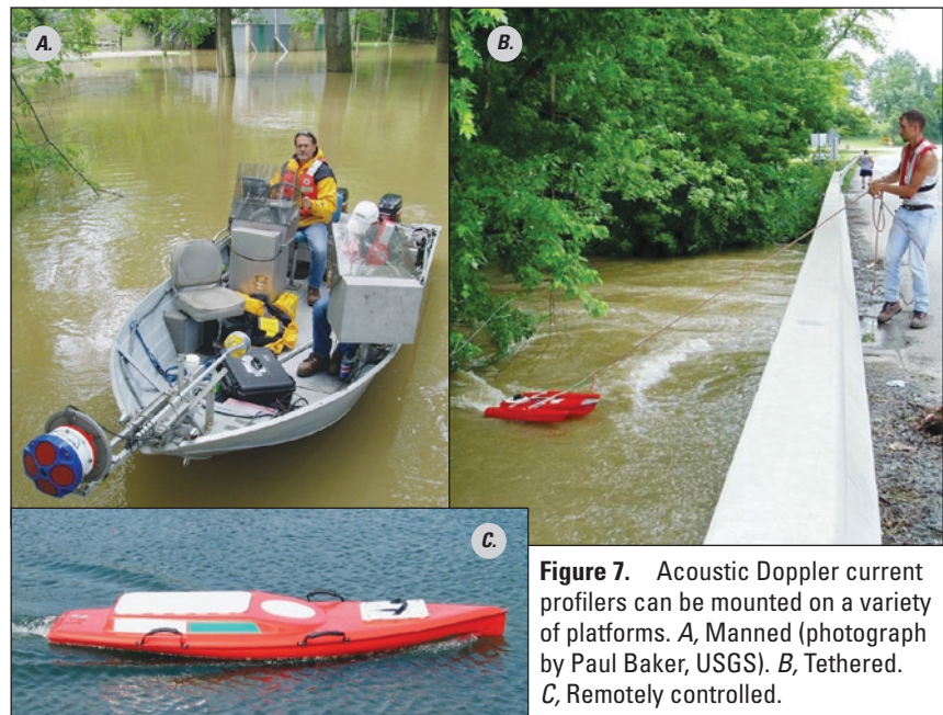
Figure 6. River discharge measured using an acoustic Doppler current profiler mounted on a boat.
