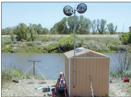
Figure 8. Ultra-high frequency (UHF) and microwave radar system can measure the surface velocity of a river.
