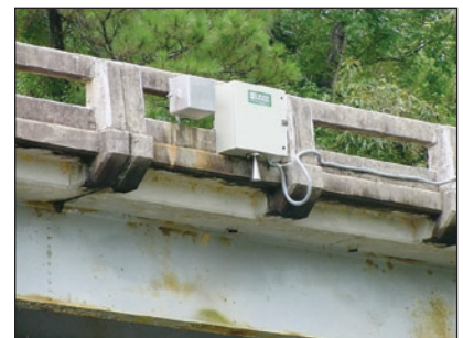
Figure 3. Stage can be measured using a non-contact radar stage sensor mounted on a bridge.
