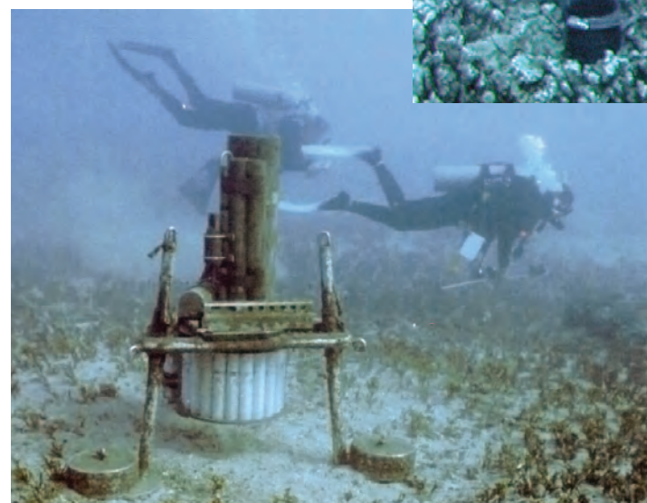
Figure 3. Time-series sediment trap at 11.5-m (37.7 ft) water depth off Kamiloloa.
