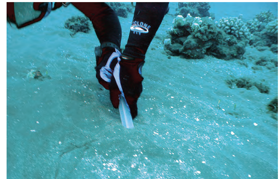
Figure 2. Diver conducting porewater extraction on the sea floor using a syringe with an aquarium airstone attached.
