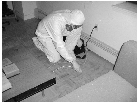
Collecting dust samples at a NYC residence after September 11, 2001
