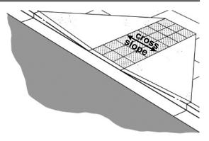
The gutter is the part of the street that borders the curb. To measure the gutter slope, place the level in the same position as the arrow in the illustration, with one end where the gutter meets the ramp and the other end towards the street. The gutter slope is parallel to the ramp and perpendicular to the curb. The gutter may slope up to 5 percent towards the curb ramp, but not more.
