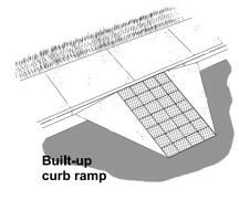
Built-up curb ramps cannot project into the path of cars. The "path of cars" includes anywhere cars are allowed to drive, including roadways, parking lot driveways, parking spaces, and access aisles.
