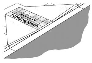
to the ramp run and perpendicular to the curb, shows where to measure the running slope.
