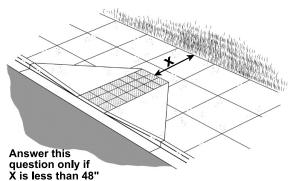
Place the level in the same position and location as each of the arrows in the illustration to the left. The slope of the curb ramp's flared sides may not exceed 8.33 percent when there is less than 48 inches between the top of the curb ramp and the edge of the sidewalk at the other side ("**x**").
