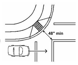
When taking this measurement, the measuring tape should be aligned parallel to the ramp run itself and should stretch from the intersection of the ramp and gutter to the innermost edge of the pavement marking.
