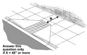
To measure the slope of a curb ramp's flared side, place a level on the flared side near the edge of the curb. The level should be placed so that it is parallel to the curb. Place the level in the same position and location as each of the arrows in the illustration to the left.
