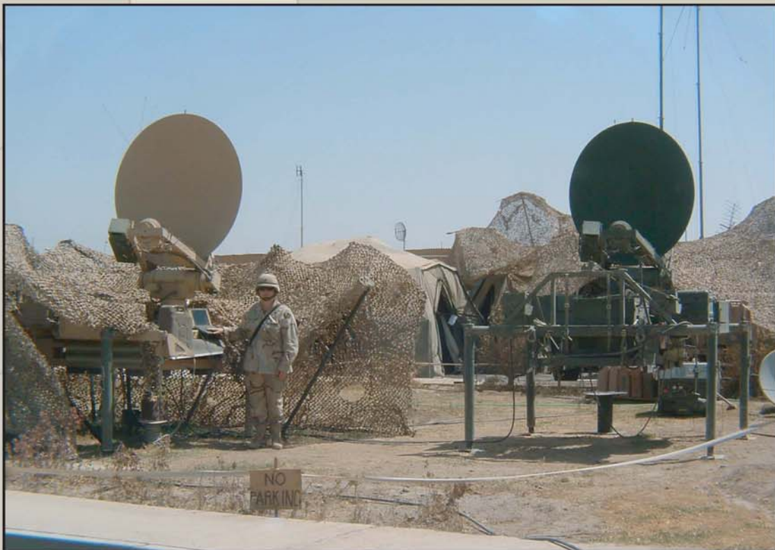
Two SMART-T Terminals outside an Operations Center
