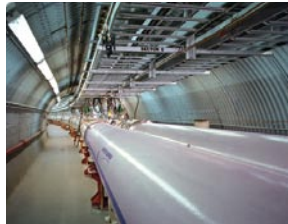
RHIC's two rings are made of 1,740 superconducting magnets, which focus and steer the beams.
