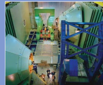
The PHENIX detector examines entities such as photons, electrons, and muons, in addition to the particles tracked by STAR. PHENIX stands for Pioneering High-Energy Nuclear Interacting Experiment.
