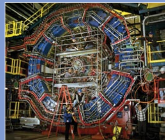
The STAR detector tracks and analyzes thousands of particles, such as protons, neutrons, and pions, that may be produced in each collision inside the detector — as seen in the cover image. STAR stands for Solenoidal Tracker at RHIC.
