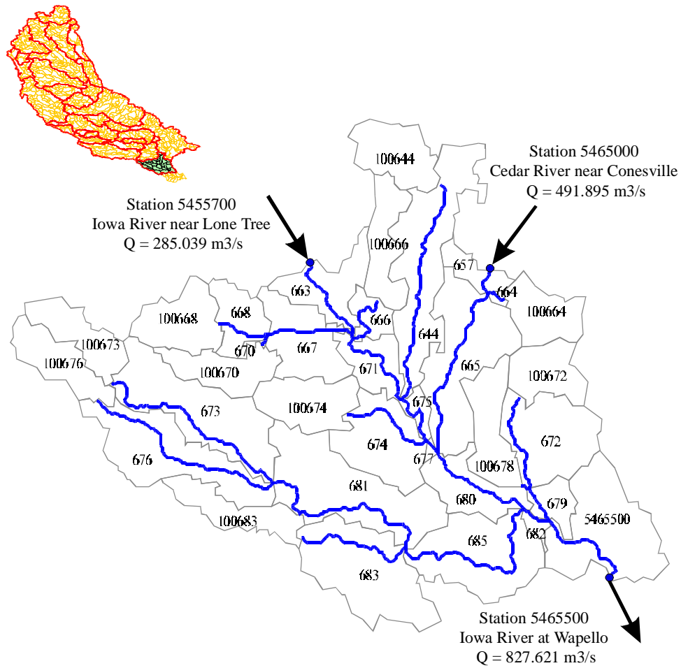
Figure 4.18 Location of the gauged zone 5465500, its subdivision into modeling units, and the USGS gauging stations.
