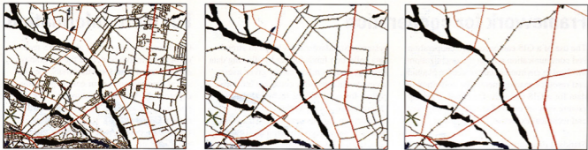
Figure 3b, c, d. These digital maps of Boone County, N.J., are all at a scale of 1:500,000. The information content of the maps has been reduced through the process of generalization in two stages, from 1:100,000 scale on the left to 1:250,000 scale in the center, then from 1:250,000 scale to 1:500,000 scale on the right.
