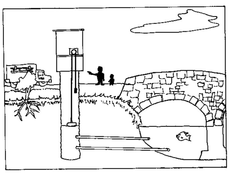
"There are pipes connecting the gage house with the river. So the level of the water in the well below the house is the same as the water in the river."
