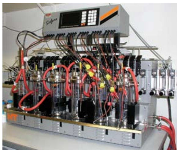
A group of six small fermentors allows researchers to grow quantities of fungi under the same conditions or to test multiple parameters simultaneously, vastly increasing the speed of conducting fungal experiments.
