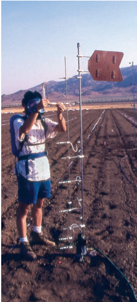
Measuring fumigant concentration at several distances above the soil surface, a student adjusts the rate of airflow through a charcoal sample collector. The charcoal is used to absorb and trap fumigant gases, which are then analyzed in the laboratory.
