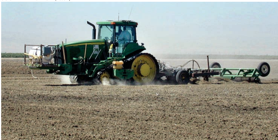
A tractor is used to inject Telone II into the soil at a depth of 46 inches. Following the tractor is a disk and ring roller—used to compact the soil and close any fractures, thus reducing emissions to the atmosphere.
