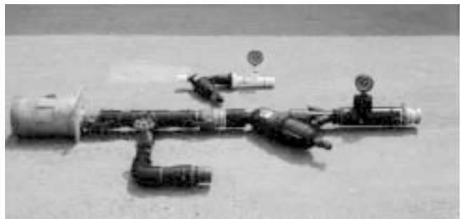
Screen filters, pressure regulators, and pressure gauges
